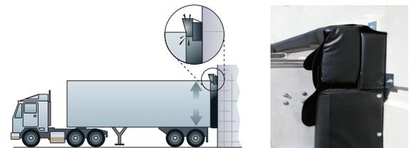
*WearMaster's 4" exposure wear panels move with the trailer, extending fabric life in key wear areas.*
