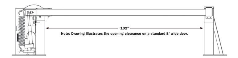
DGB-M (Manual Activation) Counter-balanced steel arm with steel supports, Dampened arm return
